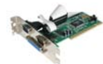
2Port 16550 Serial and 1Port EPP/ ECP Parallel Slot Saver PCI Card PCI2S1P
